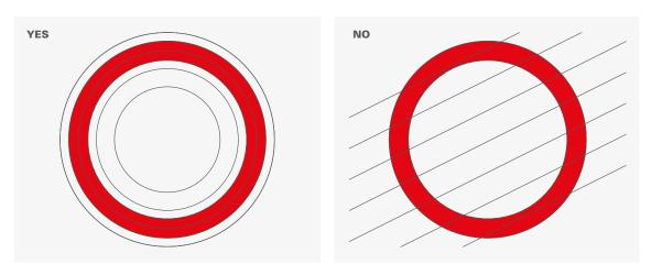
If, however, circular machining is not possible, reasonable sealing performance can be obtained if surface roughness is <Ra  $0.8 \mu m$ .
