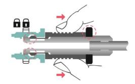
**4.3.** To unmate the SV plug, untighten the knurled ring to unlock and pull the outer sleeve of the plug:
