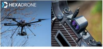
Hexadrone SAS, a French company specializing in the mechatronic development of solutions linked to the use of civil and military drones, equips its multi-functional, modular drone called Tundra with a Fischer UltiMate<sup>™</sup> USB 2.0 connector that is waterproof, reliable in all conditions and suitable for intensive use in the field.
