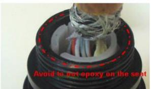
Slide down one Washer and fit it into the seat of the Body.
