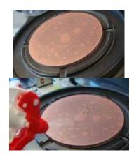
Clean the polishing pad with demineralized water and lint-free cloth, from the center outwards.
