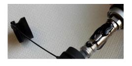
Apply epoxy on the Shrink Tube "K" and slide the Bend Relief "L" until the end of the Bend Relief "L" abuts the Rear Nut "J".
