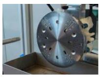
Wipe abundantly the polishing tool holding the termini with demineralized water and clean it carefully with a lint-free cloth.
