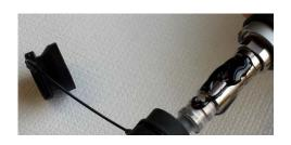
Apply epoxy on the Shrink Tube "J" and slide the Bend Relief "K" until the end of the bend relief bottoms against the Back Nut "I".
