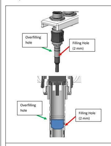
Slowly inject the epoxy inside the Potting Set Body "F" using the filling hole located at the bottom of the Potting Set Body "F".
