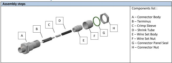
Note: the pictures shown in this section represent a R03 receptacle. The following assembly steps are valid for R01 receptacles as well.
