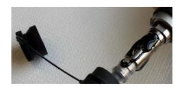
Apply epoxy on the Shrink Tube "H" and slide the Bend Relief "I" until the end of the Bend Relief "I" bottoms against the Back Nut "G".
