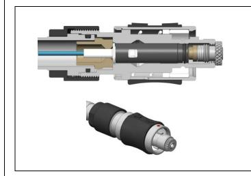
Screw the Sleeve Holder "A" in the Connector Body "B" until the Sleeve Holder "A" is free to rotate.
