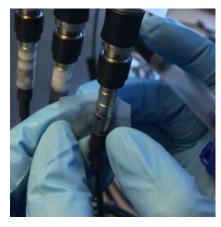
Remove any excess epoxy from the assembly (if any), apply tape on both filling and overfilling holes and place the assembly onto the curing oven block. Curing time: 12 hours @ approx. 23 °C
