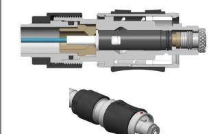
Screw the Sleeve Holder "A" in the Connector Body "B" until the Sleeve Holder "A" is free to rotate.
