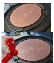
Spray some demineralized water on the polishing pad and place the polishing film, starting at edges of the polishing pad.
