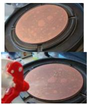
Clean the polishing pad with demineralized water and lint-free cloth, from the center outwards.
